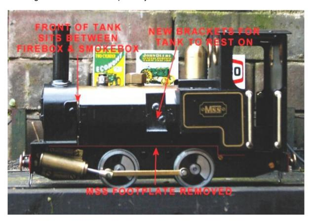
Remove the fittings that originally were used for mounting the tank and fold the bottom edges of the tank upwards.
