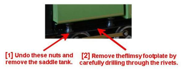
Then remove the flimsy footplate that the tank was bolted to.
