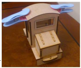
Assemble the two parts of the buffer/couplings in place and insert in the locating hole in the buffer beam
