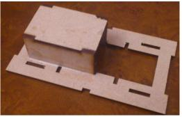
Glue two sloping sides to the cab back (The cab front and back are handed, the front has an additional slot in it for the control panel).
