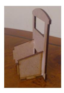
Locate the cab back over the battery box onto the loco floor
