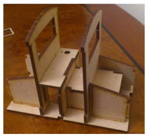
Glue the cab sides in place. Use clamps or elastic bands to hold the assembly in place while the glue sets
