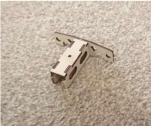
Attach the stretcher bar side plates into one of the side frames for each bogie, (you may need to sand the end a little to fit).
