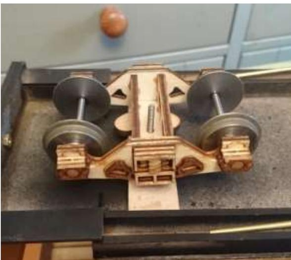
Place the inverted bogie over the pivot bolt
