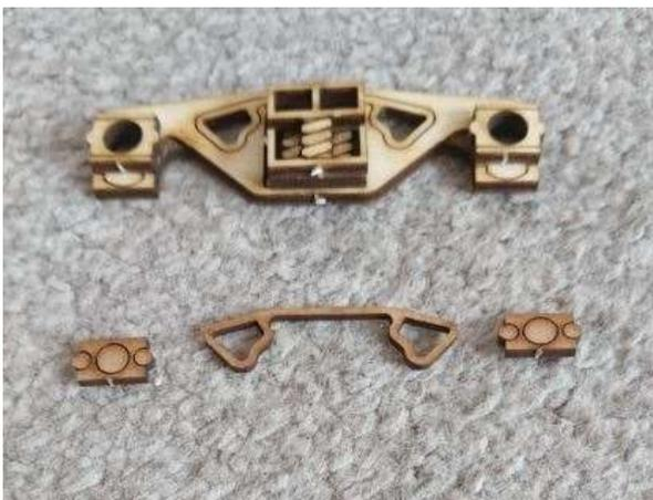
The last step in this section is to glue the 1.5mm axle box covers and frame strengthener onto the side frame
