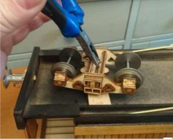
Secure the bogie in place with the 3mm nut using pliers or nut runner if you have one.
