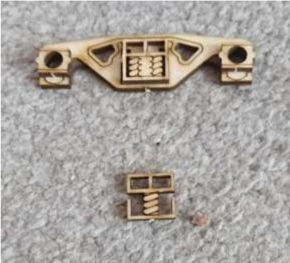
First glue the axle boxes and the double spring parts onto the side frame
