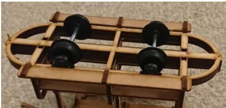
Slide the axle boxes onto the ends of the axle and glue the axle boxes into the wagon frame. Ensure no glue comes into contact with the axle ends or wheels
