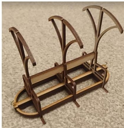
Glue the second end frame in place. Then apply glue to the centre frame.
