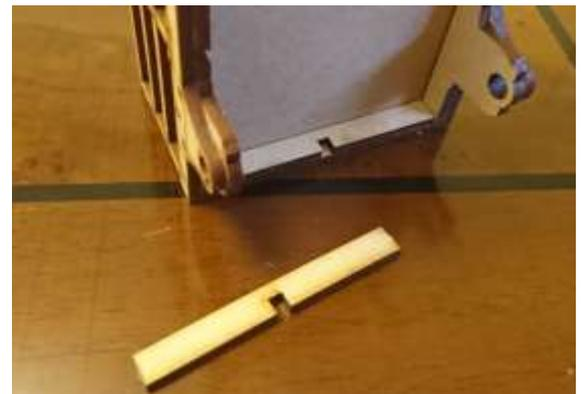
Insert the centre cross beams into the slots in the sole bars, again with the central slot facing away from the wagon floor
