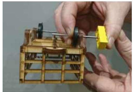
Glue together either two or three of the dumb butters to match your desired coupling height, form the brass pin into a hook shape and insert into the hole through the coupling and final mount the assembled buffer on the wagon above the coupling beam
