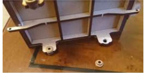
At this point test the axles for free running in the bearings. If the axle bearings are even slightly misaligned the axle could be very stiff to turn. DON'T PANIC!
